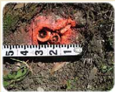
A pincushion corner where three monuments set by land surveyors all ostensibly represent one corner position. What service is being provided here that could not be provided by the cheapest expert measurer?
