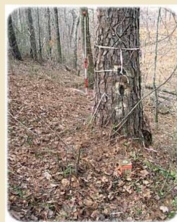
A pincushion corner where two monuments, more than 20 feet apart, represent one section corner. The monument in the background (a pipe next to the prism pole) was identified as a property corner when the landowner bought her property in the early 1950s. Then, in the 1980s, a contractor working for the forest service came along and set a "new corner" by proportionate measurement (the monument in the foreground). Again, what valuable service is being offered that cannot be provided by the cheapest expert measurer?
